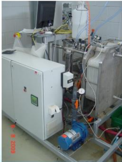
Test unit in Jeddah, Saudi-Arabien . Brine concentration.
